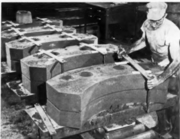
From 75 to 80 gear segments are made each day by Riverside Foundry, Bettendorf, Iowa, for a leading earth moving equipment manufacturer. Two \text{CO}_2 -hardened halves are assembled to make a mold weighing 750 lb. Accuracy of the process has eliminated the machining of gear teeth
